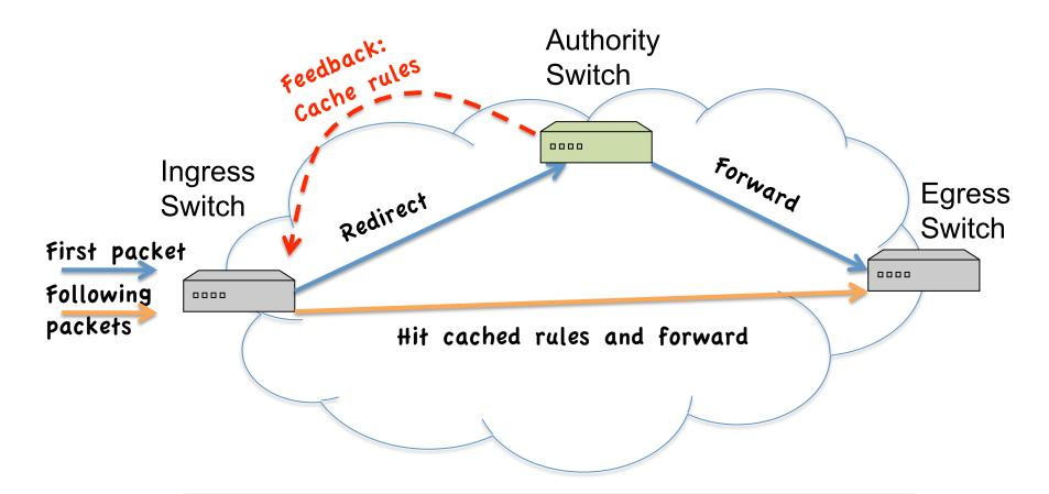
A slightly longer path in the data plane is faster than going through the control plane
